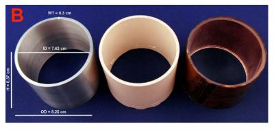
Fig. 1. (Left) Master Al filter with its outlined dimensions. (Middle) Custom casted Er-based filter for our low energy scans. (Right) A Cu filter used for our high-energy scans.
