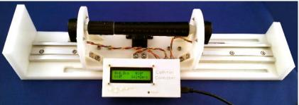
**Figure 1.** Master input device is shown. Encoders detect imposed motion from manual manipulation of the black handle. Position information is processed in real-time and then streamed to a slave robot.
