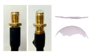
Figure 1 showing transducers with flat and convex matching layers and their respective 3D renderings.
