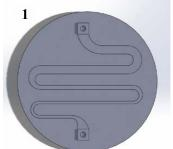
**Figure 1.** A CAD drawing of the mold to be CNC milled for the production of PDMS microfluidic chips
