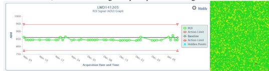
Figure 1. (a) ROI signal in a daily uniformity phantom (b) Peak variance deviation of daily uniformity phantom
