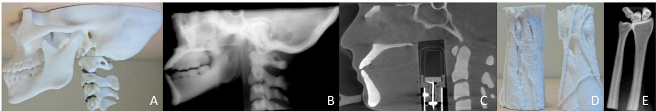
Figure 1. Maxillofacial phantom: Assembled internal 3D printed parts including mandible, spine (C1-C4 vertebrae with intervertebral discs) and maxilla. (A) Planar x-ray image acquired at 80kV. (B) Sagittal CBCT image with 6cc ion chamber inserted. (C). Forearm phantom: 3D printed forearm muscle printed with white resin modified by adding glass bubbles. (D) Planar x-ray image acquired at 60kV. (E)
