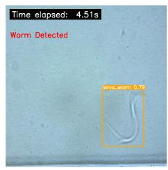
Figure 2: Larva worm Detected with YOLOv5 model
