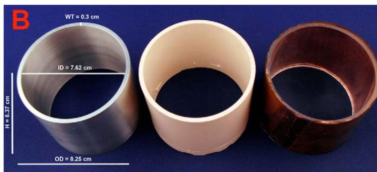
Fig. 1. (Left) Master Al filter with its outlined dimensions. (Middle) Custom casted Er-based filter for our low energy scans. (Right) A Cu filter used for our high-energy scans.
