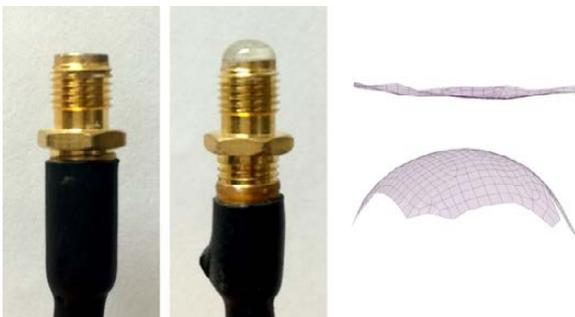
**Figure 1** showing transducers with flat and convex matching layers and their respective 3D renderings.
