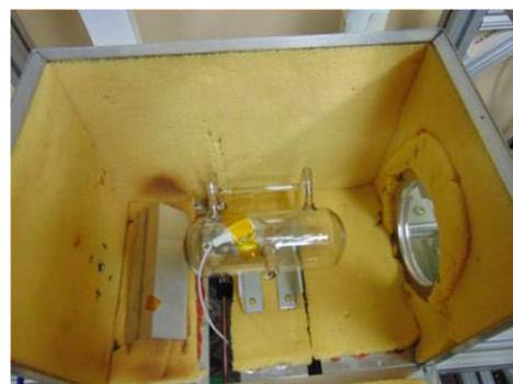
**Figure 2.** The cell of the custom-built polarizer
