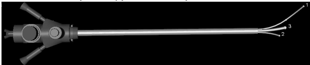
**Figure 1.** Virtual neuroendoscope with three continuum tools being designed.
