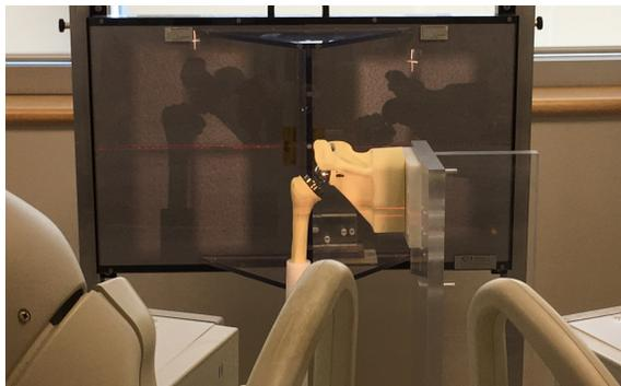
**Figure 1:** RSA imaging setup: two x-rays from different foci expose two radiograph cassettes; a calibration cage lies in front of the cassettes.
