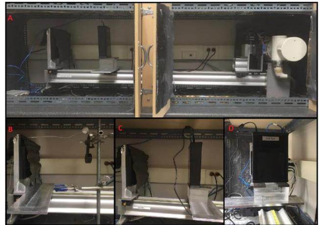
**Figure 1:** A) X-ray Detector (far left), prototype (middle), X-ray tube (far right). B) X-ray Detector (left), Ion Chamber (right). C) X-ray Detector (left), prototype (right). D) Frontal view of the clinical prototype.
