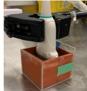
Figure 1. Temporal-enhanced ultrasound acquisition setup. The clamp holds the transducer in place on the phantom surface.
