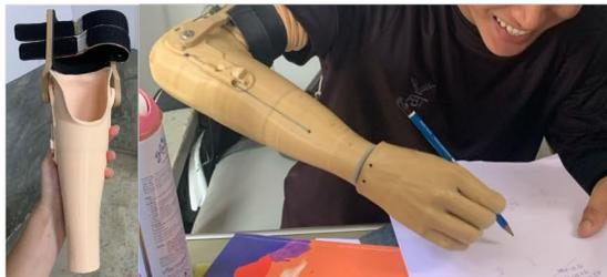
Fig 3: Left: Printed short below-elbow prosthetic. Right: Recipient testing their fitted prosthetic.
